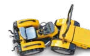
EOS V5.65 AR ISODIAMETRIC, MONODIRECTIONAL OR REVERSIBLE, WITH CENTRAL ARTICULATION
