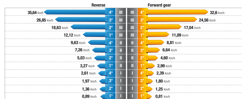
GRAPH OF SPEEDS IN KM/H OF THE AR AND RS VERSION TRACTOR
